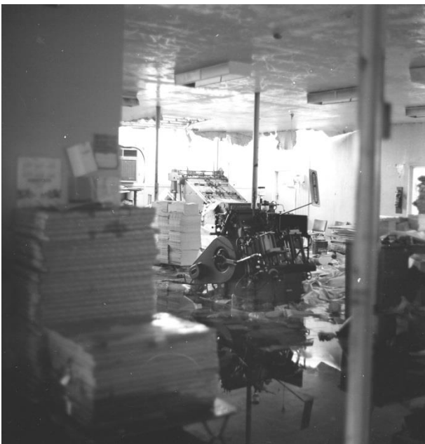
A view from the compositing area. The machine in the foreground is a new Heidelberg Platen Press. The machine at the rear of the picture is one of two Selecta flat-bed presses.
