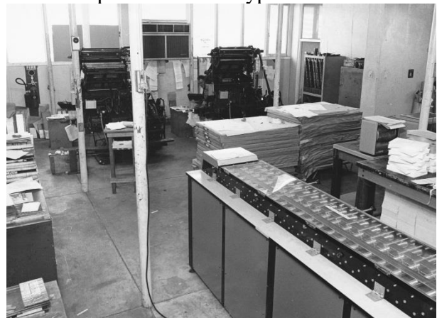
The equipment on the right was a 30 bin collator to be used collate documents such as Hansard . Early December 1974
