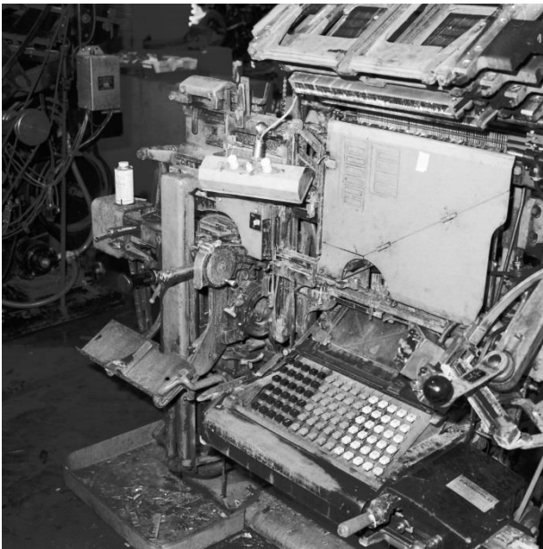
↑ One of the Intertypes with a Fairchild tape-reader attached.
