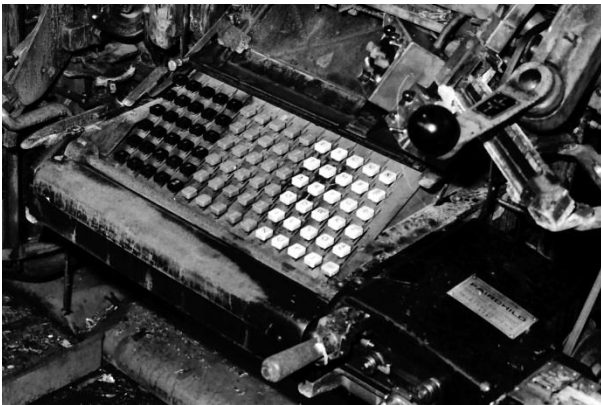
Fairchild tape reader attached beneath the keyboard of the Intertype.
