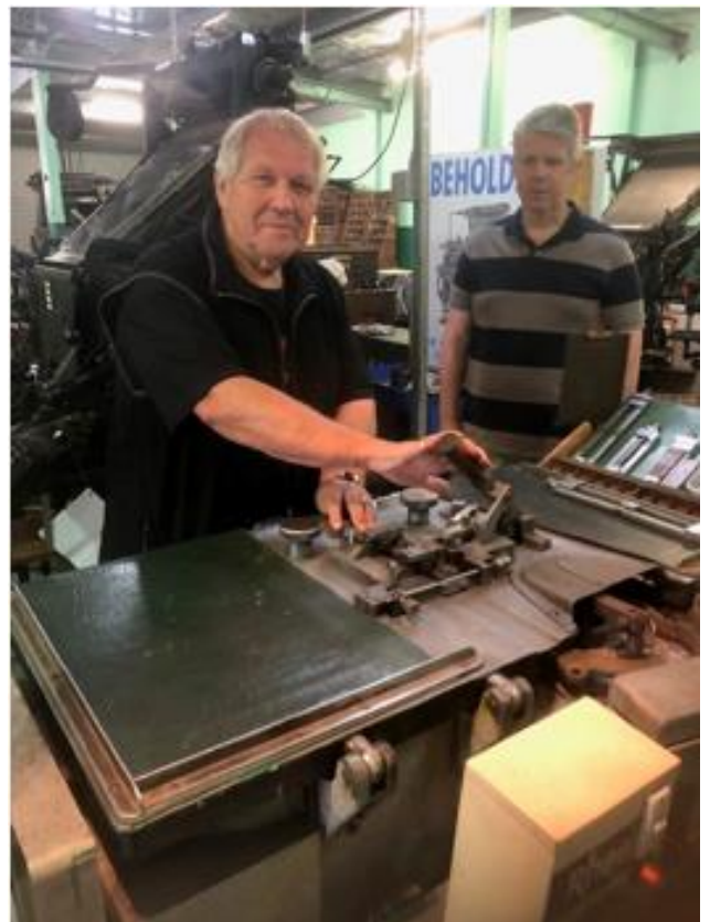
Lionel Morris – checking the set up and casting the slug on the Ludlow watched by son Robert
