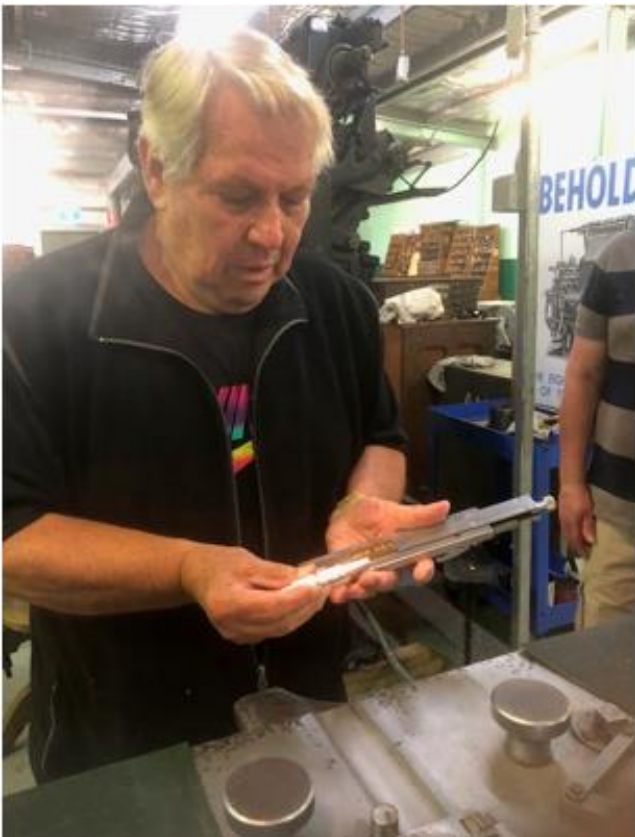
Lionel Morris – checking the set up and casting the slug on the Ludlow watched by son Robert
